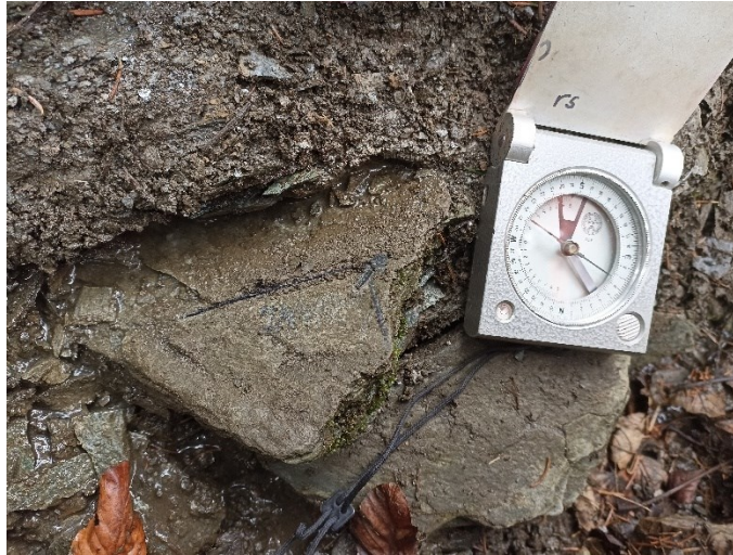
Figure 28: Taking samples for a petrophysical analysis in the laboratory. Using a geological compass, the orientation of the sample can be transferred to the laboratory.
