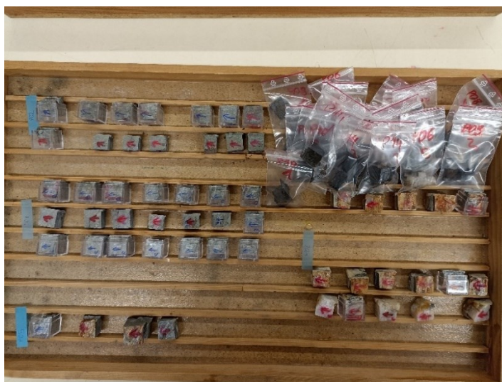
Figure 29: Specimens (2x2 cm) from different sampling points and pulverized samples in small bags.
