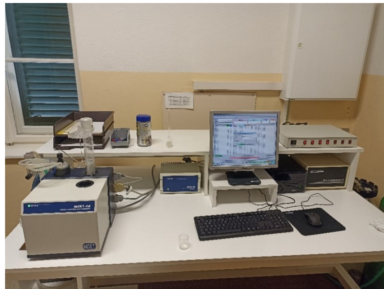
Figure 30: Kappabridge MFK1-FA from Agico for measuring the susceptibility and the curie temperature.
