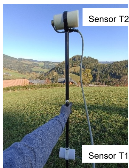
Figure 25: Proton precession magnetometer GSM-19T from GEM Systems. The two sensors filled with kerosene are 1 m and 2 m above the ground.
